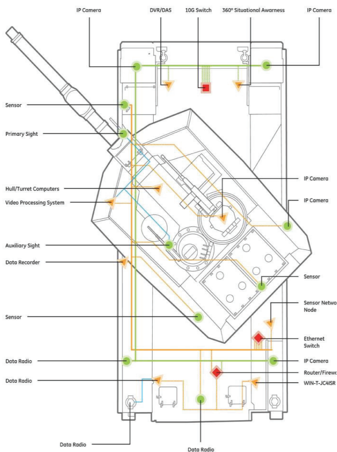
Fig. 4. Vetronics for a main battle tank [17]
